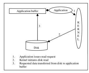
Figure 4: Reads under Direct I/O
