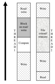
**Figure 7:** Inode serialization under Concurrent I/O on JFS2
