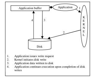
Figure 5: Writes under Direct I/O
