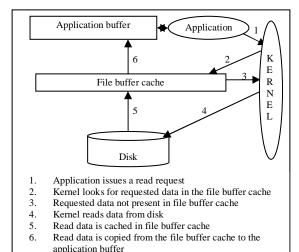
Figure 2: Reads under cached I/O - buffer cache miss
