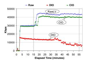
**Figure 9:** Disk I/O throughput (in kilobytes of data transferred per second) over run duration.
