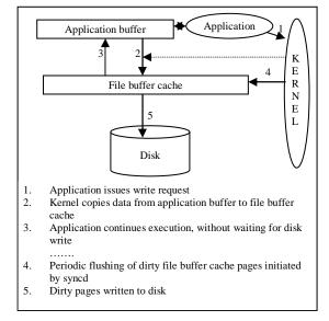
Figure 3: Writes under cached I/O
