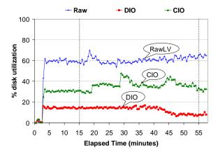
Figure 10: Highest disk utilization over run duration.
