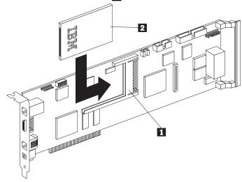
7. Connect one end of the token ring cable 2 to the PCMCIA connector on the PCMCIA card 1 as shown in the following figure.
