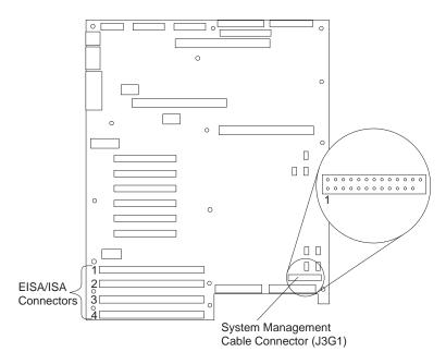
Figure 7. PC Server 704 System Board
