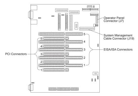
Figure 1. PC Server 325 Models 8639-EJ0, ES0, ESV, RS0, EM0 System Board
