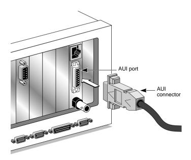
Figure 2-4 Connecting the 3C509B-COMBO NIC Using the AUI Port
