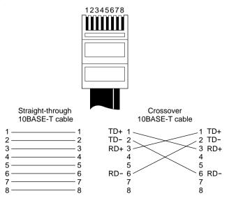
Figure 5-2 Straight-through and Crossover Cable Pinouts
