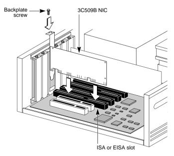
Figure 2-1 Inserting the 3C509B NIC in a PC
