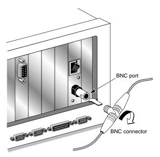
Figure 2-3 Connecting the 3C509B-TPC NIC Using the BNC Port
