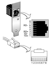
Figure A-1 RJ-45 Connector Pin Assignments
