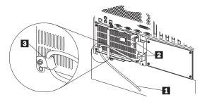
Plug the power cord into a properly grounded electrical outlet.
