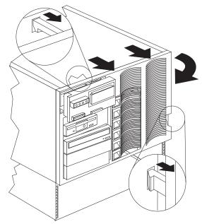
a. While releasing the top and side bezel tabs, rotate the left side of the bezel away from the system.
