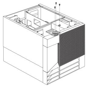
Remove the interior LED and speaker assembly mounting screws. then; remove the interior LED and speaker assembly.
