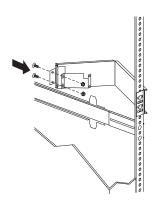
Installing the server in a rack: You will use eight screws (M4 by 8).
