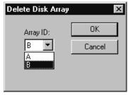
2. Select the desired disk array ID from the pull-down list.
