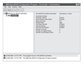
Click on the icon on the Tool Bar to switch from the Information mode to the Configuration mode.
