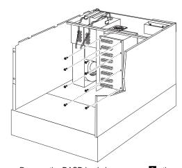
a. Remove the DASD backplane screws 1, then; remove the DASD backplane.
