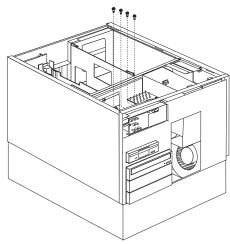
a. Remove the information panel LED assembly screws, then; remove the assembly.
