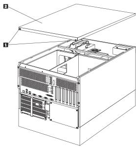
8. Loosen the four thumbscrews **1** at the rear of the shuttle.
