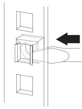
Attach a slide-bracket assembly to the front of the rack:
