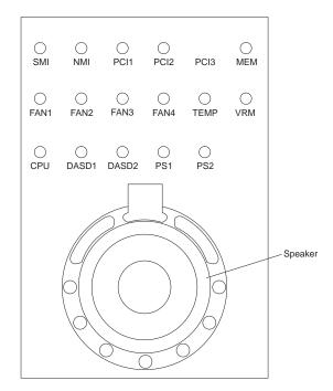
To replace the diagnostics panel LEDs, you must replace the interior LED and speaker assembly, see "Interior LED and speaker assembly" on page 217.
