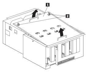
Processor housing coverQuarter-turn fasteners
