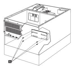
b. Remove the power backplane cover screws 1, then; remove the power backplane cover.
