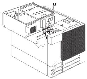
Secure the air diffuser 1 in the server by positioning the air diffuser on the matching metal tabs 2 on the shuttle.
