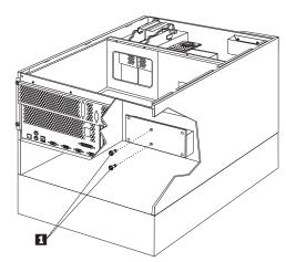
a. Remove the power backplane screws **1**, then; remove the power backplane.
