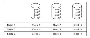
A hard disk failure within the array results in loss of data in the logical drive assigned RAID level-0, but *only in that logical drive*. If you have logical drives assigned RAID level-1 or level-5 in the same array, they will not lose data.
