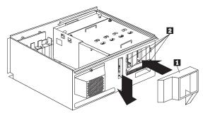
Seat the shuttle in the server and tighten the four shuttle thumbscrews.
