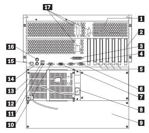
PCI Expansion Slots: The server has six peripheral component interconnect (PCI) expansion slots. Four of the PCI slots support hot-plug PCI adapters.
