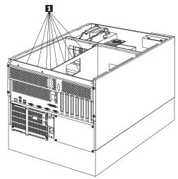
4. Remove the processor board screws 11, then; lift the processor board out of the tray.
