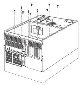
a. Remove the system board mounting screws, then; remove the system board.
