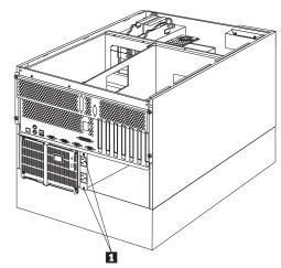
3. Remove the voltage regulator card mounting screws 1, then; slid the voltage regulator card out of the server.
