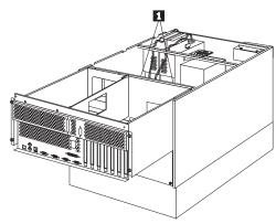
a. Remove the power backplane cover screws 1.
