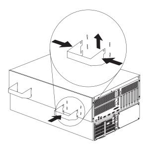
10. Lift the server from the slide bracket assemblies and place the server on a flat, nonconductive surface.
