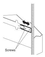
Insert screws (6M by 16 mm) through the mounting rail to the slide-bracket assembly. Do not tighten the screws.
