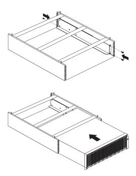
Removing cage nuts: Device installation might require the removal or moving of the rear-pane cage nuts. If you need to move the cage nuts, follow this procedure to move them and then go to "Installing cage nuts" on page 234 to install them in the correct position.
