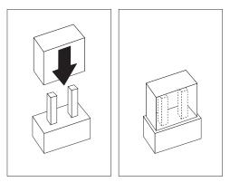
Align one of the holes in the bottom of the jumper with one of the pins on the pin block, and then slide the jumper carefully onto that pin only.
