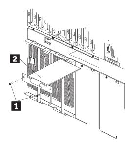
To remove the power control card, do the following:
