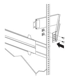
c. Position the server bracket on the cable-management arm.
