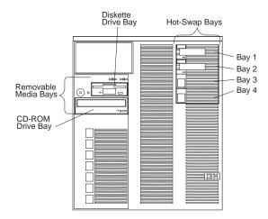
Your server contains hardware that lets you replace a failed hard disk drive without turning off the server. Therefore, you have the advantage of continuing to operate your system while a hard disk drive is removed or installed. These drives are known as *hot-swappable* drives. They are also referred to as hot-swap drives.
