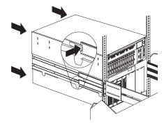
Attach the cable-management arm to the server using the captive screws.
