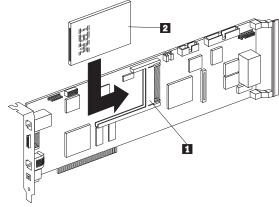
Connect one end of the token ring cable 2 to the PCMCIA connector on the PCMCIA card 1 as shown in the following figure.
