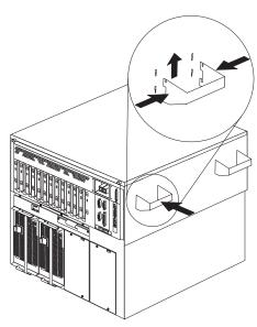
10. Lift the server from the slide bracket assemblies and place the server on a flat, nonconductive surface.
