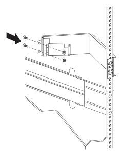
**Installing the Server in the Rack:** In this section, you will use eight screws (M4 by 8 mm) and four screws (M6 by 16 mm).
