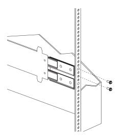
5. Attach the other slide-bracket assembly to the front and rear of the rack.
