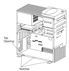
c. Insert the bottom cover tab into the tab opening.
