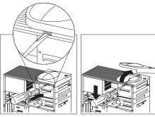
Remove the top-handle screw and the screw from the drive-support bracket that holds the upper drive cage in place. Then, move the drive cage towards the power supply until it stops, and lift it out of the server.
