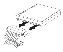
3. Remove the visible screws that hold the drive and slide it out the front of the server.
