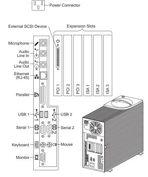
Power Connector: The server power cable connects here.
