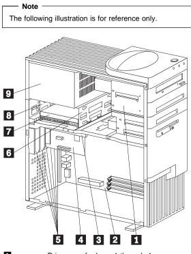
Drive cage for bays 1 through 4 System board Riser card Adapter Expansion slots Drive cage for bays 5 and 6 Bay 6, hard disk drive Bay 5 Power supply
