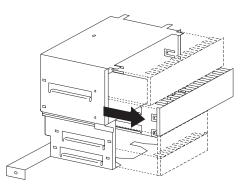
2. Touch the static-protective package containing the new drive to any *unpainted* metal surface; then, remove the drive from it.
