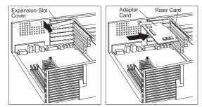
8. Install the bracket and the screw.
