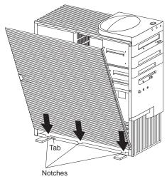
d. With one hand, align the top so that the cover rests against the server. With the other hand, press the cover at the bottom left corner, above the left rotated foot.
