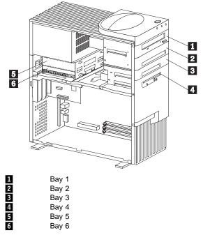
The drives in bays 5 and 6 must have nonremovable media. (In some models, the server comes with a hard disk drive in bay 6.) To install or remove drives in these bays, you must remove the rear (lower) drive cage.
