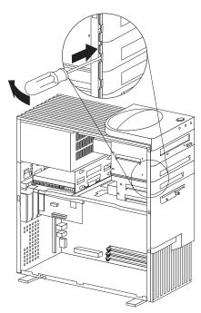
If knockouts are present in the drive bay opening, twist them with a screwdriver or pliers to remove. The following illustration shows the type of knockout in bays 2 and 3.
