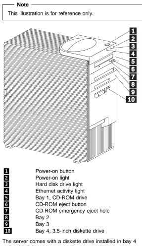
and a CD-ROM drive installed in bay 1. If the server comes with a hard disk drive, it is installed in bay 6.
