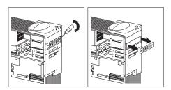
3. Install the drive in the bay opening and secure the drive by inserting screws.
