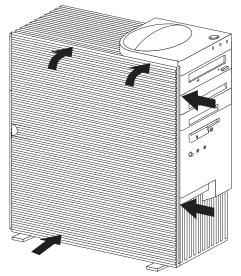
e. Keep the hand at the top to hold the cover in place. Use the thumb from the other hand to slide the cover forward, as shown in the following illustration. Make sure that the cover is latched into position.
