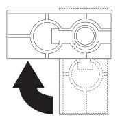
When you need to access the inside of the server to install options, you might find it easier to place the server on its side, so that the system board is facing you. If you do so, rotate the feet in towards the server, so that they do not detach due to the weight of the server.
