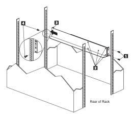
Loosen the five screws (four large screws and one small screw)
