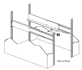
Remove the two small 6-32 screws on the interior side of the rails. Save these screws to install the Expansion Unit
