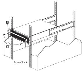
2. Remove screws 2 and remove bezel 1.
