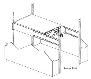
1. Remove screws 1 from assembly rails at rear.
