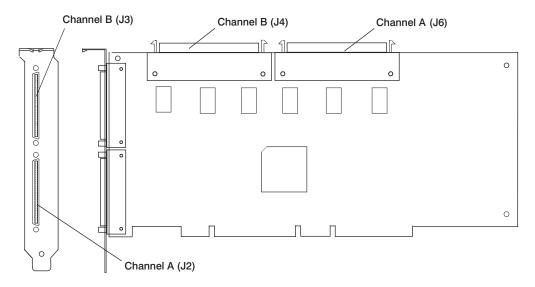
**Note:** The adapter has built-in SCSI terminators on each channel that are automatically enabled when a cable is attached to either the external or internal connector.
