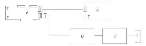
**Note:** A converter cable may be used to attach VHDCI connectors on the adapter and P-shell connector on external cables. The terminator may be built into the last device or it may be externally attached.
