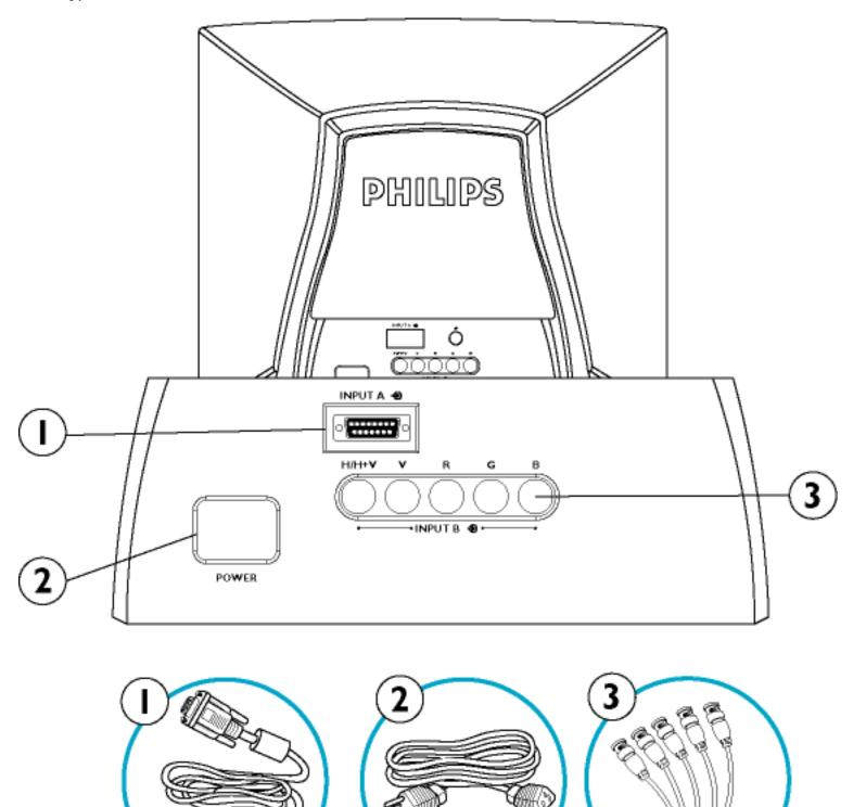
**1.** D-Sub Port - Attach the D-Sub connector that comes with your monitor here. Other end connects to your PC.
