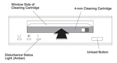
Figure 2. Loading the Cleaning Cartridge
