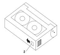
Figure 3. Setting the Write-Protect Switch
