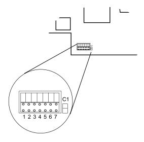
To set a SCSI address, you must install jumpers onto pin positions 1, 2, 3 or 4 on the jumper block of the interface bridge card. Table 2 on page 10 shows the jumper placement necessary to set each position to On or Off. To set a position to On, insert a jumper onto both the top and bottom pins. To set a position to Off, insert the jumper onto the top pin only.
