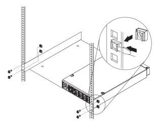
If your rack has round holes, slide the 10-32 clip nuts into place on the rear of the rack.
