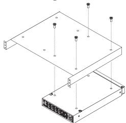
5. Turn the tray over so that the hub is on top of the tray.
