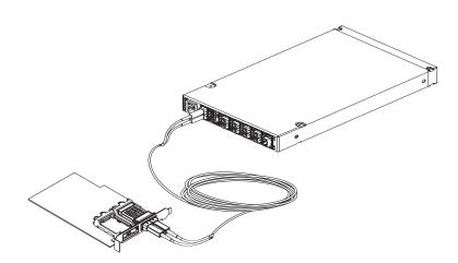
The IBM Fibre Channel Hub is a 7-port central interconnection for Fibre Channel Arbitrated Loops that follow the ANSI FC-AL standard. Each Fibre Channel Hub port receives serial data from an attached node and retransmits the data out of the next hub port to the next node attached in the loop. Each reception includes data regeneration (both signal timing and amplitude) supporting full-distance optical links.
