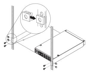
7. Pick up the tray and line up the top and bottom screw holes with the clip nuts on the rack. While holding the tray in place, install four of the larger screws.
