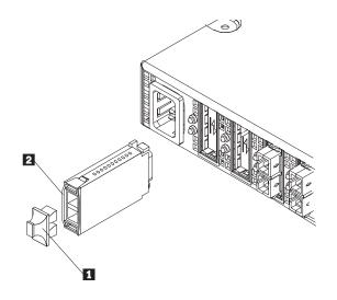
2. Insert the cables into the GBIC.
