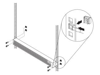
If your rack has round holes, use the 10-32 clip nuts and hex washer headed screws.
