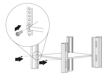
7. Hold the shelf level and line up the threaded hole on one side of the rear of the shelf with a hole in the rear mounting rail.
