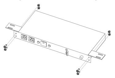
The bottom two side braces on both sides of the rack are installed with a vertical clearance (distance) of 51.3 cm (20.2 in.) to accommodate the PDU installation. If the braces do not have this clearance, proceed with step 2. If the braces have this clearance, go to step 3 on page 3.
