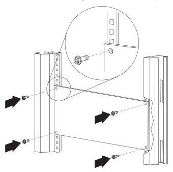
5. Tighten the four screws.
