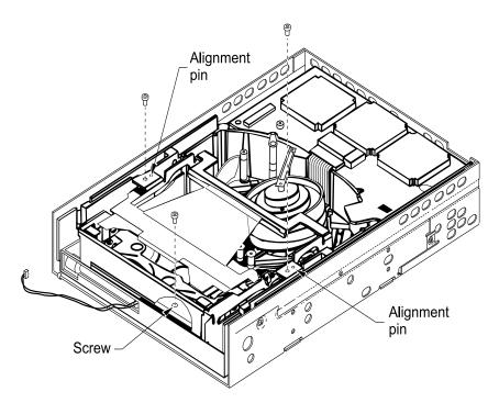
Figure 6 Installing the cartridge loader
