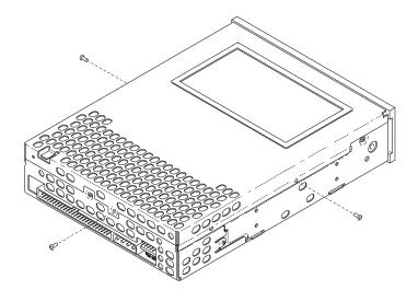
Figure 9 Replacing the top cover
