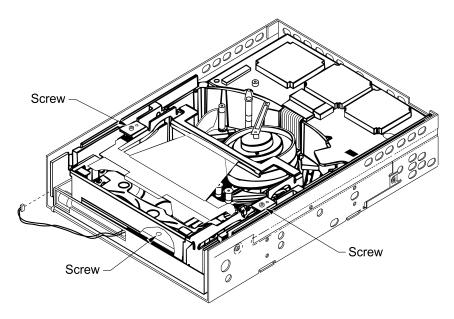
Figure 5 Removing the cartridge loader screws and disconnecting the wires
