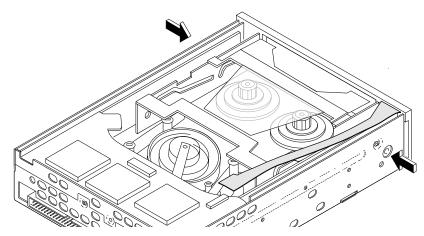
Figure 3 Removing the faceplate
