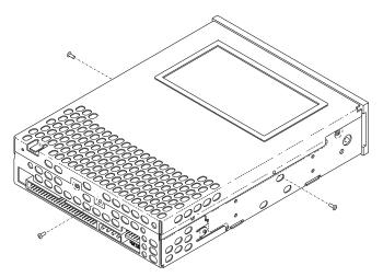
Figure 1 Removing the top cover
