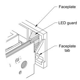
Figure 7 Positioning the faceplate
