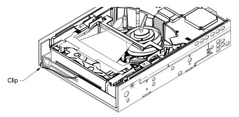
Figure 4 Loosening the cartridge loader wire clip
