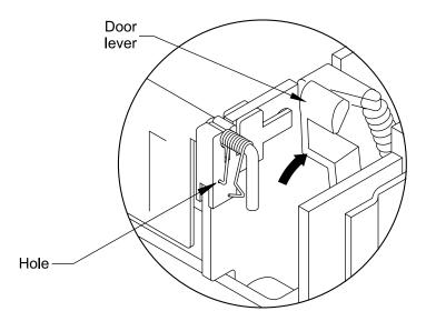
Figure 10 Repositioning the door lever and replacing the spring
