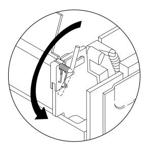
Figure 11 Tensioning the door spring
