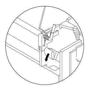
Figure 12 Pulling the door lever to the front
