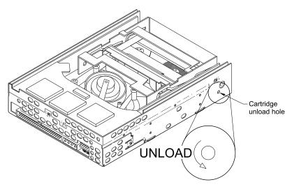
Figure 13 Readjusting the cartridge loader
