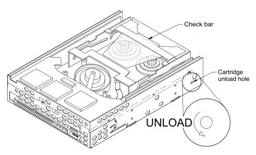
Figure 4 Adjusting the cartridge loader
