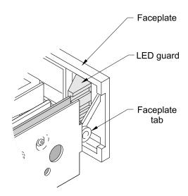
Figure 14 Positioning the faceplate
