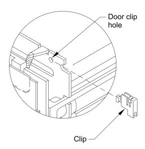
Figure 8 Replacing a door clip (left side shown)
