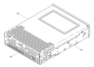
Figure 16 Replacing the top cover
