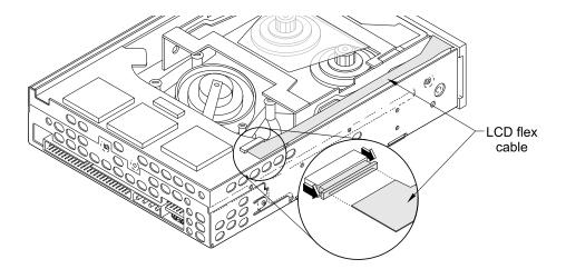
Figure 2 Loosening the LCD flex cable connector
