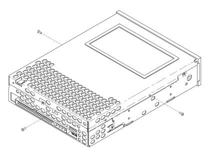
Figure 1 Removing the top cover
