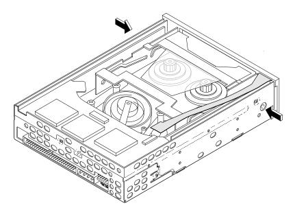
Figure 3 Removing the faceplate
