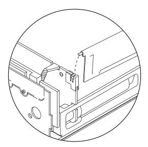
Figure 9 Inserting the left end of the hinge pin into the door clip
