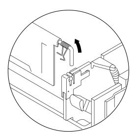
Figure 7 Removing the right hinge pin
