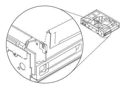
Figure 5 Removing the left hinge pin
