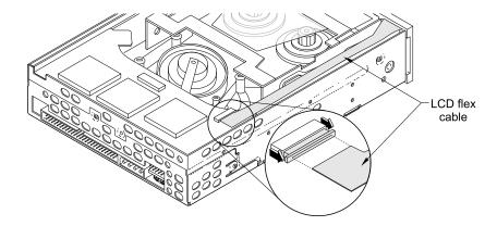
Figure 15 Loosening the tab on the LCD flex cable connector
