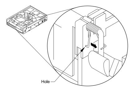
Figure 6 Removing the left end of the spring
