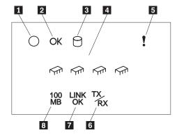
System Power Light: When this green light is on, system power is present in the server. When this light flashes, the server is in standby mode (the system power supply is turned off and AC current is present). When this light is off, either a power supply, AC power, or a light has failed.
