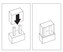
• Align one of the holes in the bottom of the jumper with one of the pins on the pin block, and then slide the jumper onto that pin only.
