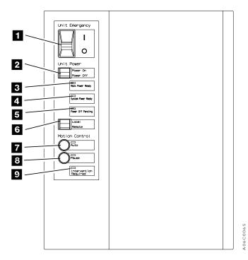
Figure 22. Operator Panel without Convenience Input/Output Station Feature
