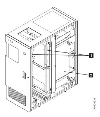
Figure 12. Model HA1, Left Service Bay Functional Components (Right-Front View)
