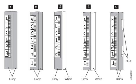
Figure 17. Cartridge System Tape Labels
