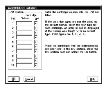
Figure 122. Insert Unlabeled Cartridges Window
