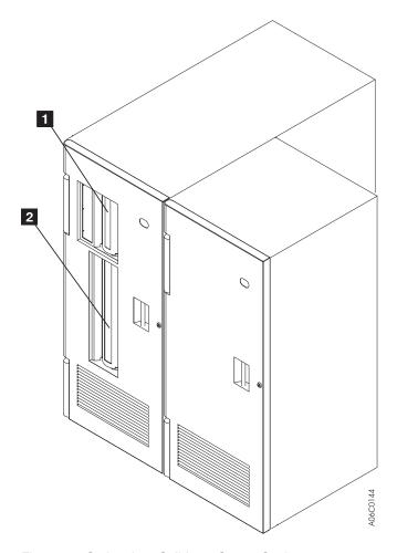
Figure 35. Optional 30-Cell Input/Output Station
