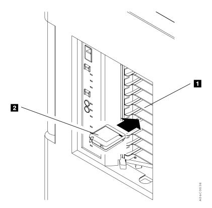
Figure 34. Inserting Cartridges in the Convenience Input/Output Station
