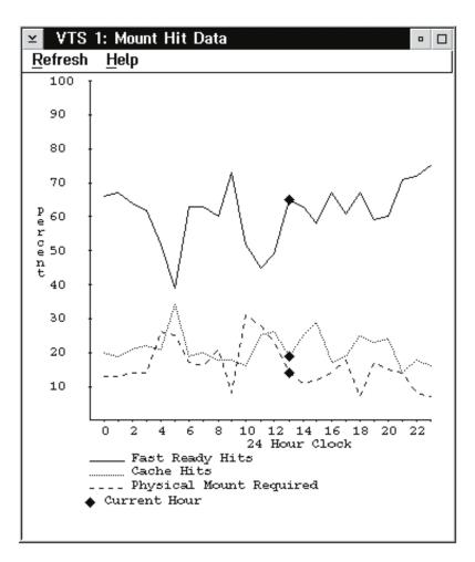
Figure 73. VTS Mount Hit Data Window
