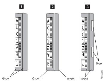
Figure 15. Cartridge System Tape Identification
