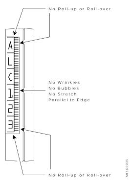
Figure 18. Cartridge Label Position
