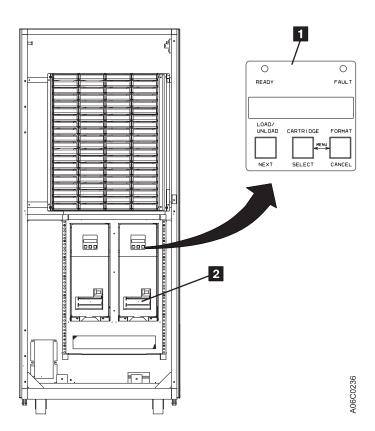
Figure 26. 3490E Controls and Indicators for Model F1A
