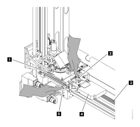
Figure 149. Cartridge Removal from the Gripper
