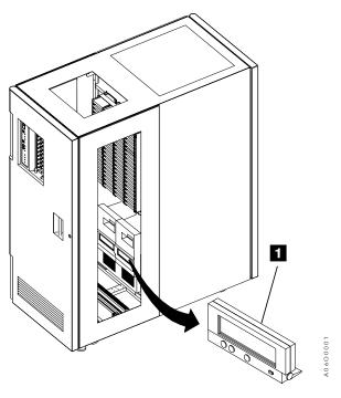
Figure 27. 3590 Model B1A and E1A Operator Panel
