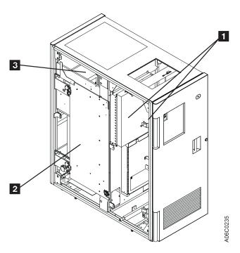
Figure 13. Model HA1, Right Service Bay Functional Components (Left-Front View)
