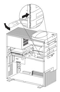
2. If knockouts are present in the drive bay opening, twist them with a screwdriver or pliers to remove.
