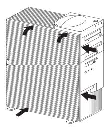
e. Keep the hand at the top to hold the cover in place. Use the thumb from the other hand to slide the cover as shown in the following illustration. Make sure that the cover is latched into position.
