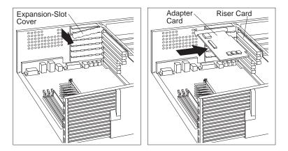
8. Install the bracket and the screw.
