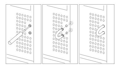
4. If you have completed installing the U-bolt and do not want to install any other internal options, replace the server side cover and reconnect all external cables and power cords. (See "Completing the installation" on page 148 if you need additional information.)
