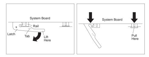
7. Using the tab, slide the system board out and set it aside.
