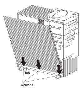
d. With one hand, align the top so that the cover rests against the server. With the other hand, press the cover at the bottom left corner, above the left rotated foot.
