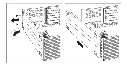
5. Slide the tabs on the end of the cover out of their openings and remove the cover.
