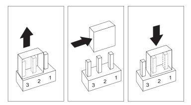
11. After clearing CMOS memory, you must reconfigure the server. After reassembling the server (see "Completing the installation" on page 148), use the Configuration/Setup Utility program to reset the date and time, reset any passwords, and reconfigure
