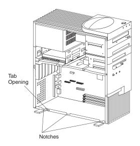
c. Insert the bottom cover tab into the tab opening.
