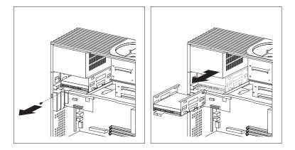
3. If you are removing a drive, remove the screws that hold the drive in the bay assembly and slide the drive out of the bay assembly.
