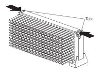
3) Lift the microprocessor out of the connector.
