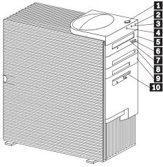
Your server comes with a diskette drive installed in bay 4 and a CD-ROM drive installed in bay 1. If your server comes with a hard disk drive, it is installed in bay 6.
