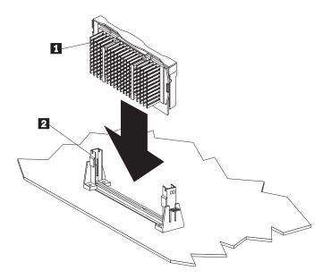
If the microprocessor has tabs at the upper corners instead of an adapter with a handle, press inward on the retainer tabs until they click into place.
