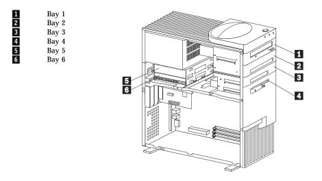
The drives in bays 5 and 6 must have nonremovable media. (In some models, the server comes with a hard disk drive in bay 6.) To install or remove drives in these bays, you must remove the rear (lower) drive bay assembly.
