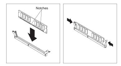
*Note:* Adding or removing DIMMs changes the configuration information in the server. When you restart the server, the system displays POST error 164. Start the Configuration/Setup Utility program and select **Save Settings**.
