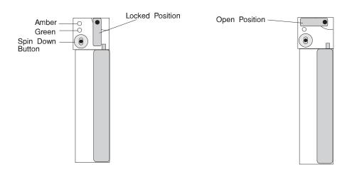
6. Disconnect the drive from the connector on the backplane, by grasping the handle on the drive tray and carefully pulling the drive out of the system. Store the drive in a safe place.
