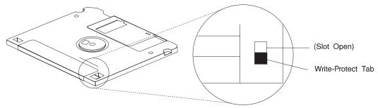
• To allow writing onto a diskette, slide the write-protect tab to cover the protect slot.
