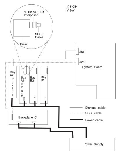
**Attention** Route the cables (SCSI-2 and power) at the rear of the media drives so they do not block airflow or bind between the fans and media drives.
