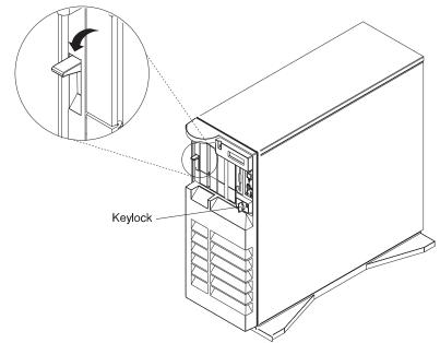
2. Reinstall the door at the front of the system by aligning the pins with the hinges, and sliding the door down.
