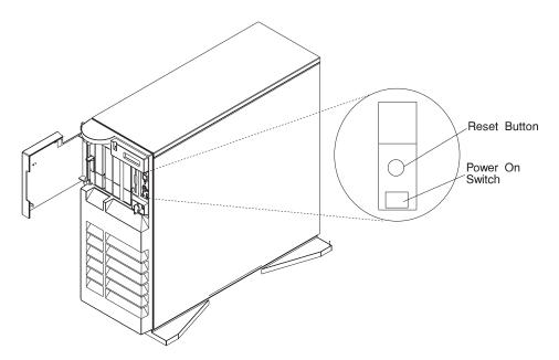
5. Check your display or ASCII terminal for configuration information displayed as the *power-on self-test (POST)* begins. The system beeps once to indicate it is working properly.
