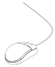
You can use the mouse to perform such functions as positioning a cursor, selecting items from a menu, or moving around in your document much easier and faster than if you used only the keyboard. The cursor moves exactly as you move the mouse on a flat surface, such as a desktop.
