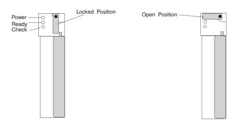
b. Position the drive carrier assembly vertically, with the connector facing the rear of the server.
