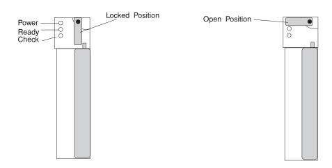
**Attention:** SSA backplanes must be fully populated. Each backplane connector must have a disk drive or a blank carrier installed at all times. If you remove a disk drive from a bay and do not replace it with another disk drive, you must install a blank carrier in that bay.
