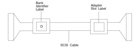
g. Connect the SCSI cable from the second SCSI internal connector to the new backplane (D or E). Refer to the following illustrations to help you connect the cables properly.
