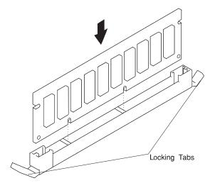
**Attention:** Inserting the memory-modules diagonally may damage the memory-modules.
