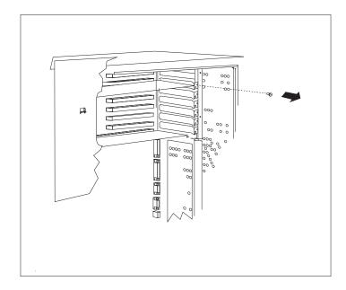
d. Carefully pull the adapter out of the system.
