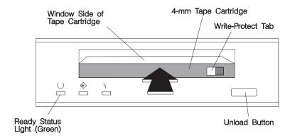
The 4-mm tape drive is ready for data operations when the tape cartridge is inserted. After the cartridge is inserted into the tape drive, the tape takes about 15 seconds to load.
