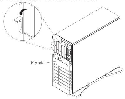
3. Reinstall the door at the front of the system by aligning the pins with the hinges, and sliding the door down.
