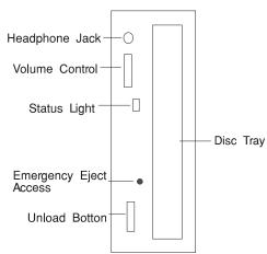
When the CD-ROM is set to On, the status light indicates one of several conditions. The following are status light states and the respective conditions of the CD-ROM drive:
