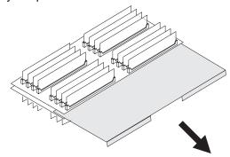
4. The card is secured in place with card retainer hooks, one on each end of the card. Open the card retainer hooks and remove the card.
