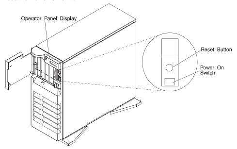
When you press the Power On switch, the Power On LED comes on and the system starts a POST (power-on self test).
