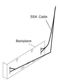
10. Connect the connector from the EPOW cable to backplane D as shown.
