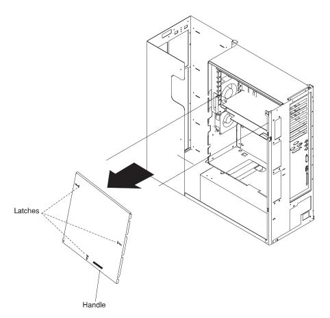
Attention If your system has the SSA bulkhead cable installed, make sure that you do not damage the cable as you remove the I/O planar cover.
