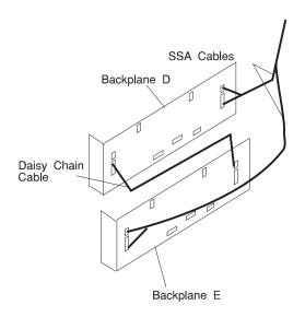
25. SSA cables connected to SSA backplanes C, D, and E is shown below.
