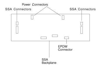
7. Attach the new power cable to backplane D.
