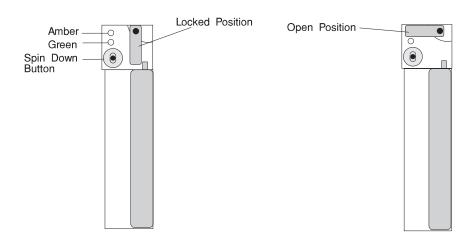
b. Position the drive carrier assembly vertically, with the connector facing the rear of the system.
