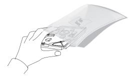
2. Check the instructions that came with the drive to see if you need to set any switches or jumpers on the drive, or if you need to attach a tray to the drive.
