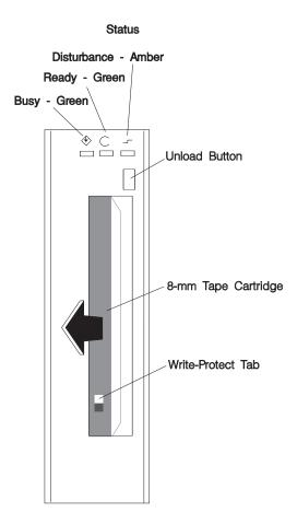
The time required for a tape to rewind and unload is between 18 seconds and 3 minutes, depending on the position of the tape when the unload button is pushed.
