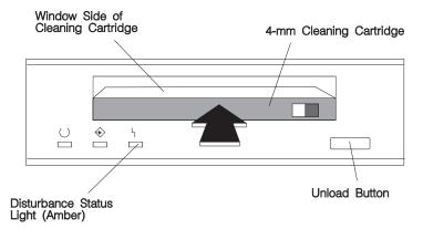
After the 4-mm cleaning cartridge has been fully inserted into the 4-mm tape drive, the following cleaning operations are performed automatically:
