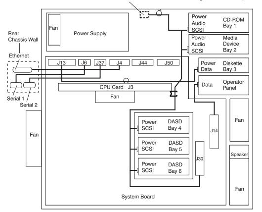
**Note:** Place the SCSI terminator through the cable clamp.
