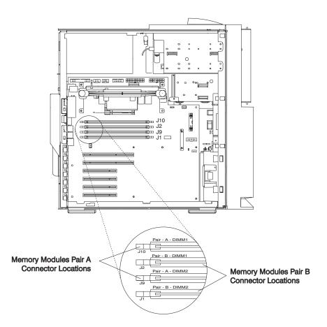
**Note:** Memory DIMMs must be installed in pairs and in the correct connector configuration. Connector ID numbers are labeled on the system board. Possible connector pair combinations are J1 and J2, J9 and J10.
