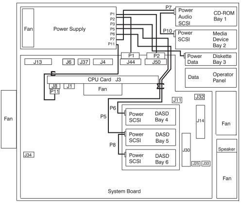
Note: If Bay 4 DASD is not installed, store the excess length of P6 cable in the cable clamp.
