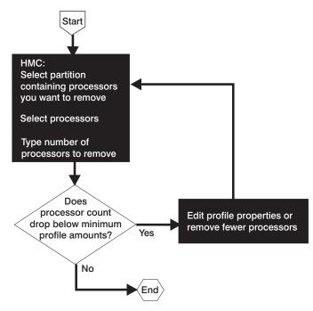
To remove processor resources from an active partition without rebooting the partition, do the following:
