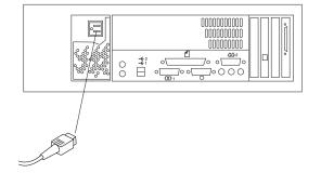
2. Plug the power cords for the monitor, HMC, and modem into electrical outlets.
