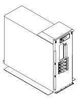
The Model 275 can be configured as a 1-way to 2-way symmetric multiprocessing (SMP) system. It has up to four disk drives and six hot-plug PCI adapters. Redundant hot-plug power supplies and cooling fans are supported.
