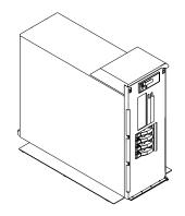
The Model 275 can be configured as a 1-way to 2-way symmetric multiprocessing (SMP) system. It has up to four disk drives and six PCI adapters. Redundant power supplies and cooling fans are supported.
