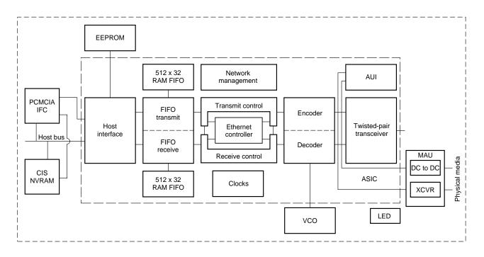
Figure 2-3. Block Diagram for PCMCIA (3C589)
