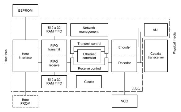
Figure 2-1. Block Diagrams for ISA, MCA, EISA (3C509, 3C529, 3C579)
