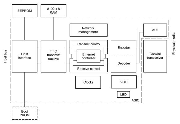
Figure 2-2. Block Diagrams for ISA (3C509B)
