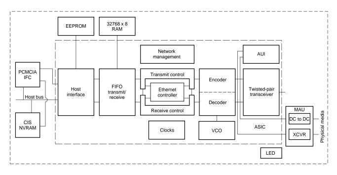
Figure 2-4. Block Diagram for PCMCIA (3C589B)
