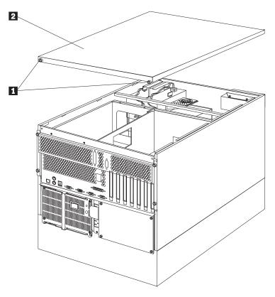
9. Loosen the four thumbscrews 1 at the rear of the shuttle.
