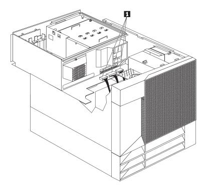
18. Secure the air diffuser 1 in the server by positioning the air diffuser on the matching metal tabs 2 on the shuttle.
