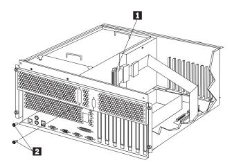
b. Remove the screws from the external connector on the bulkhead opening.
