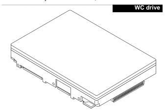
**Note:** This drive model plugs directly into a backplane connector and therefore uses no cables.
