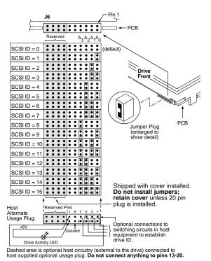
Figure 3b. Model "W" and "WC" drive ID select and LED connection
