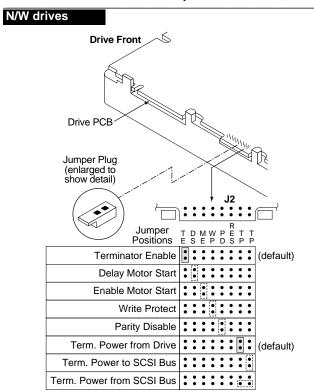
Figure 3d. Models "N" and "W" drive configurator, option select
