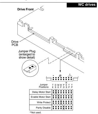
Figure 3e. Model "WC" drive configurator, option select
