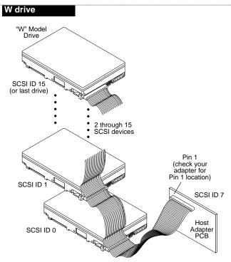
Figure 4d. Multiple-drive connection to host adapter
