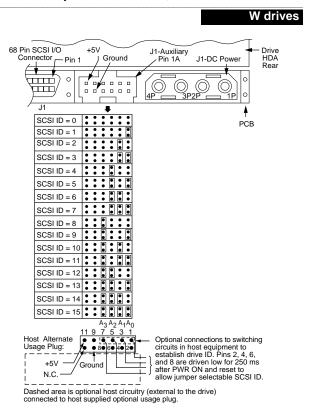
Figure 3c. Model "W" drive ID select and LED connection
