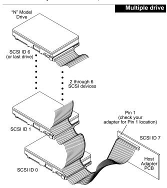
Figure 4c. Multiple drive connection to host adapter
