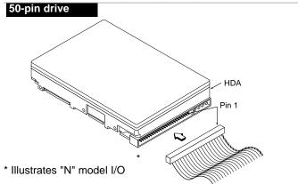
Figure 4a. Fifty-pin I/O connection to drive
