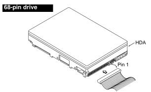
Figure 4b. Sixty-eight pin connection to drive
