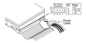
Figure 5. Power connection to drive
