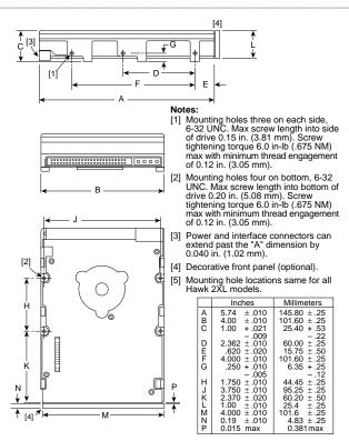
Figure 6. Mounting configuration dimensions
