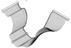
Figure 1. Two drive I/O cable
