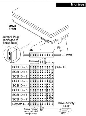
Figure 3a. Model "N" drive ID Select and LED connection
