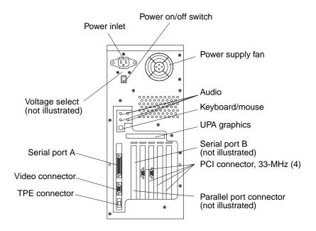
FIGURE 1-6 Ultra 10 System Unit Rear View
