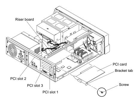
FIGURE 10-5 Removing and Replacing a PCI Card From PCI Slot 1 and/or 3 (Ultra 5)
