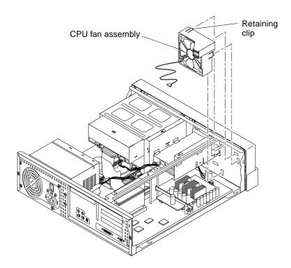
FIGURE 8-13 Removing and Replacing the CPU Fan Assembly (Ultra 5)
