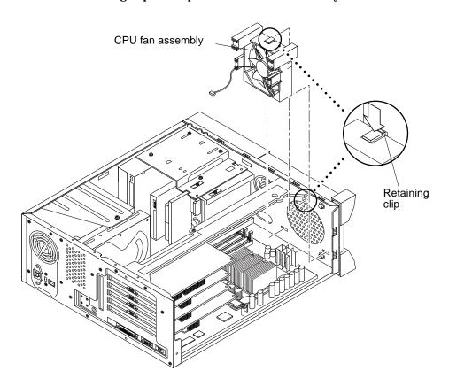
FIGURE 8-14 Removing and Replacing the CPU Fan Assembly (Ultra 10)
