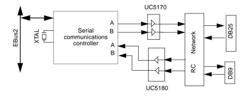
FIGURE C-13 Communications Controller Serial Ports Functional Block Diagram
