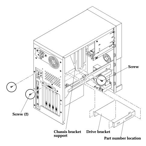
FIGURE 8-17 Removing and Replacing the Rear Drive Bracket
