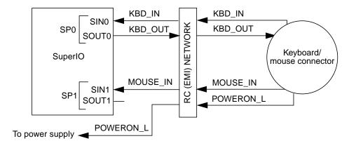
FIGURE C-12 Standard Serial Port Functional Block Diagram
