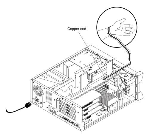
FIGURE 7-4 Attaching the Wrist Strap to the Chassis (Ultra 10)
