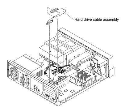
FIGURE 8-5 Removing and Replacing the Hard Drive Cable (Ultra 5)
