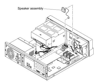
FIGURE 8-11 Removing and Replacing the Speaker Assembly (Ultra 5)
