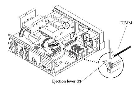
FIGURE 10-9 Removing and Replacing a DIMM (Ultra 5)
