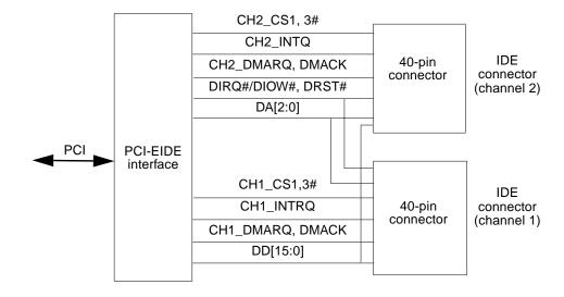
FIGURE C-4 EIDE Interface Functional Block Diagram
