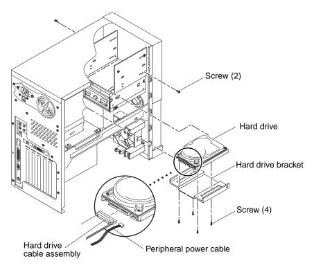
FIGURE 9-7 Removing and Replacing a Hard Drive (Ultra 10 Chassis Front)
