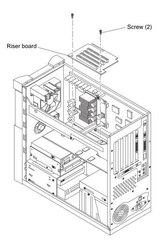
FIGURE 10-12 Removing and Replacing the Riser Board (Ultra 10)
