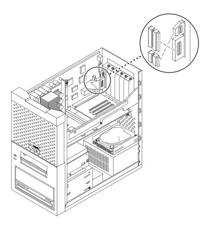
FIGURE 8-8 Removing and Replacing the Serial/Parallel Cable (Ultra 10)
