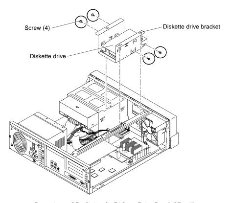
FIGURE 9-2 Removing and Replacing the Diskette Drive Part 2 (Ultra 5)
