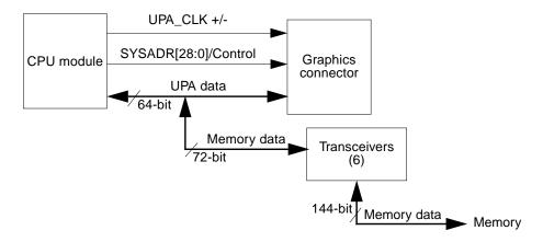
FIGURE C-2 UPA Graphics Functional Block Diagram
