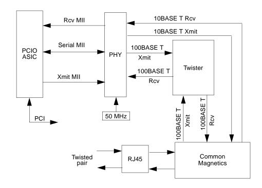
FIGURE C-3 10-/100-Mbit Ethernet Functional Block Diagram
