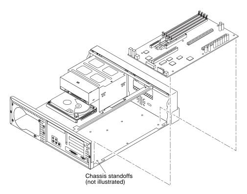
FIGURE 10-14 Removing and Replacing the Motherboard (Ultra 5)
