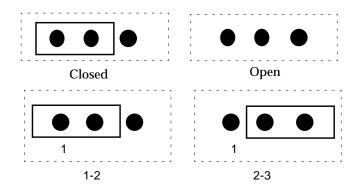
FIGURE 10-16 Identifying Jumper Pins
