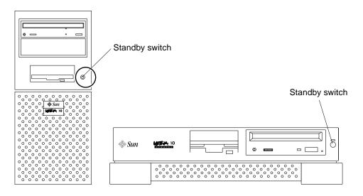
FIGURE 6-2 System Unit Standby Switch
