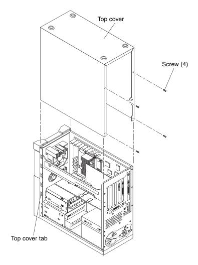
FIGURE 7-2 Removing and Replacing the Top Cover (Ultra 10)
