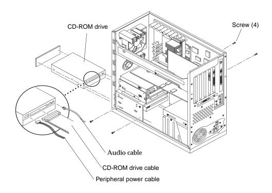
FIGURE 9-9 Removing and Replacing a CD-ROM Drive (Ultra 10)
