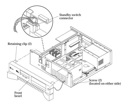
FIGURE 8-15 Removing and Replacing the Front Bezel (Ultra 5)
