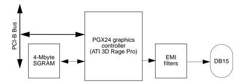
FIGURE C-9 PCI-Based Graphics Functional Block Diagram (PGX24)
