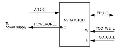
FIGURE C-14 NVRAM/TOD Functional Block Diagram
