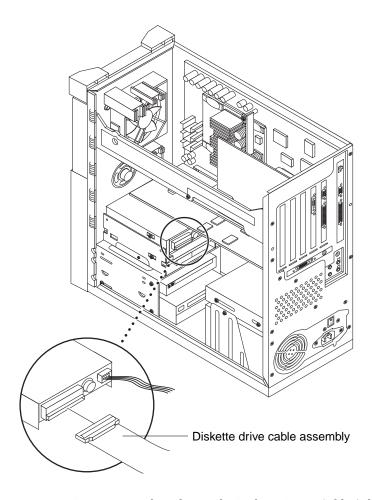
FIGURE 8-4 Removing and Replacing the Diskette Drive Cable (Ultra 10)
