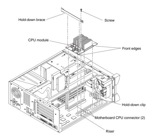
FIGURE 10-2 Removing and Replacing the CPU Module (Ultra 10)
