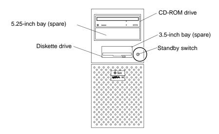
FIGURE 1-5 Ultra 10 System Unit Front View
