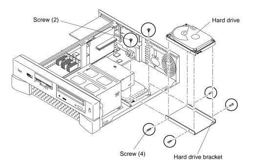
FIGURE 9-5 Removing and Replacing a Hard Drive (Ultra 5)
