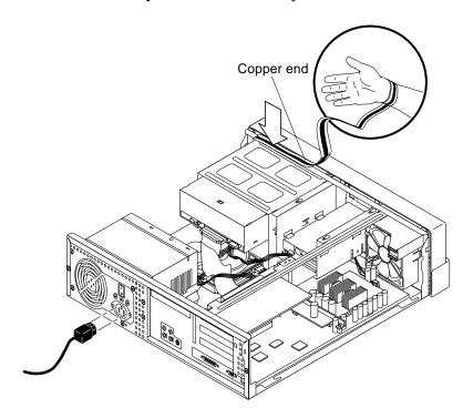
FIGURE 7-3 Attaching the Wrist Strap to the Chassis (Ultra 5)
