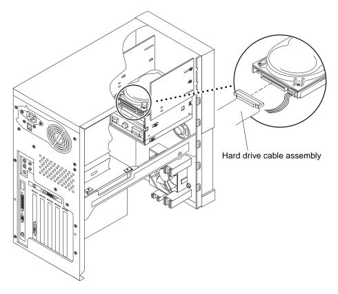
FIGURE 8-6 Removing and Replacing the Hard Drive Cable (Ultra 10)
