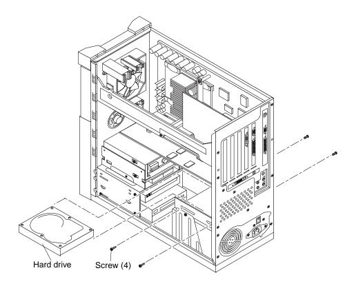
FIGURE 9-6 Removing and Replacing a Hard Drive (Ultra 10 Chassis Rear)
