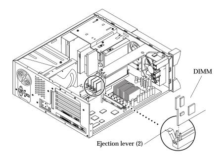
FIGURE 10-10 Removing and Replacing a DIMM (Ultra 10)
