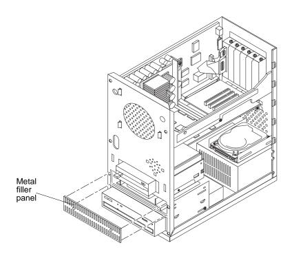
FIGURE 7-6 Removing the Metal Filler Panel (Ultra 10)
