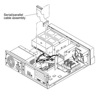
FIGURE 8-7 Removing and Replacing the Serial/Parallel Cable (Ultra 5)
