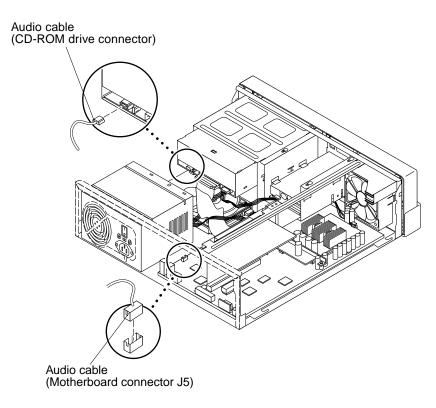
FIGURE 8-9 Removing and Replacing the Audio Cable (Ultra 5)
