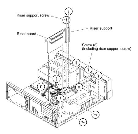
FIGURE 10-13 Removing and Replacing the Motherboard (Ultra 5)
