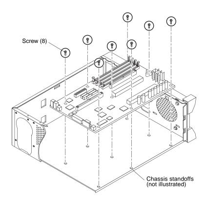
FIGURE 10-15 Removing and Replacing the Motherboard (Ultra 10)
