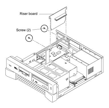
FIGURE 10-11 Removing and Replacing the Riser Board (Ultra 5)
