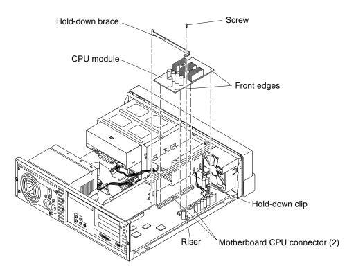
FIGURE 10-1 Removing and Replacing the CPU Module (Ultra 5)
