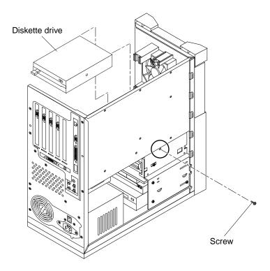
FIGURE 9-3 Removing and Replacing the Diskette Drive (Ultra 10)
