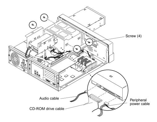
FIGURE 9-8 Removing and Replacing a CD-ROM Drive (Ultra 5)
