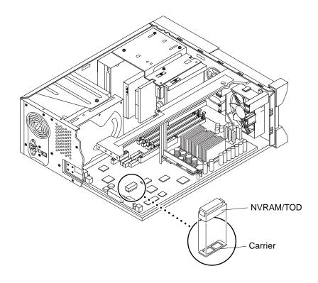
FIGURE 10-4 Removing and Replacing the NVRAM/TOD (Ultra 10)
