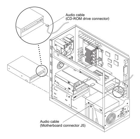
FIGURE 8-10 Removing and Replacing the Audio Cable (Ultra 10)
