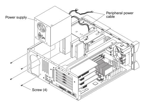
FIGURE 8-2 Removing and Replacing the Power Supply (Ultra 10))
