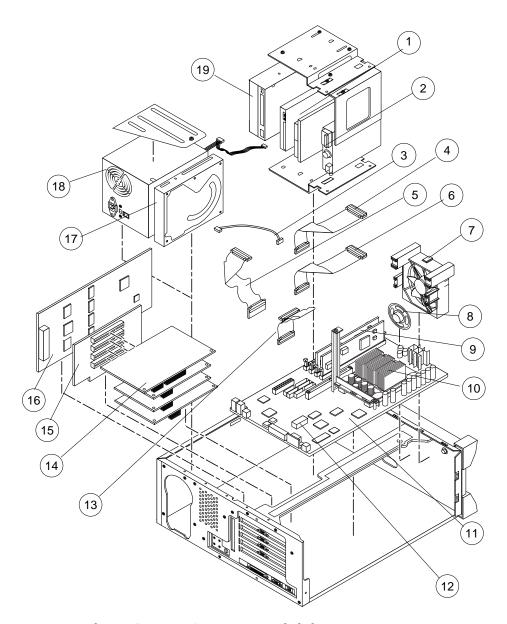
FIGURE 11-2 Ultra 10 Computer System Unit Exploded View
