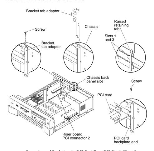
FIGURE 10-6 Removing and Replacing the PCI Card From PCI Slot 2 (Ultra 5)
