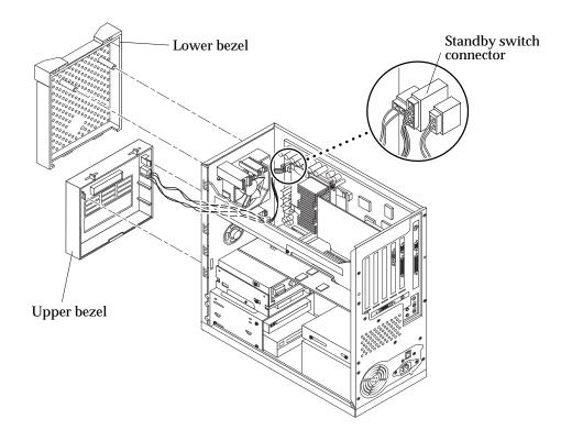
FIGURE 8-16 Removing and Replacing the Front Bezel (Ultra 10)
