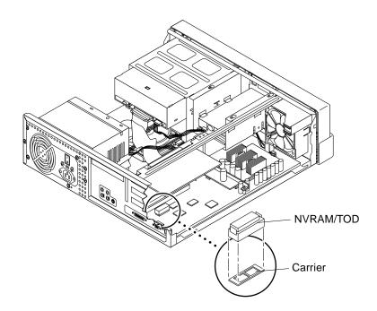
FIGURE 10-3 Removing and Replacing the NVRAM/TOD (Ultra 5)
