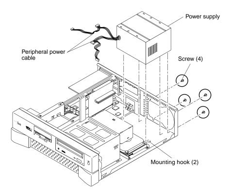
FIGURE 8-1 Removing and Replacing the Power Supply (Ultra 5)
