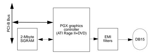
FIGURE C-8 PCI-Based Graphics Functional Block Diagram (PGX)
