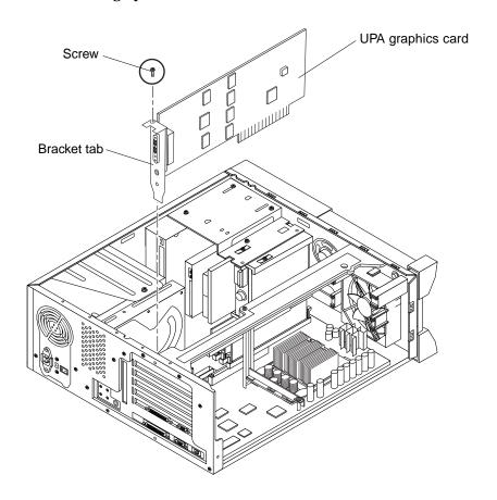
FIGURE 10-8 Removing and Replacing the UPA Graphics Card (Ultra 10)
