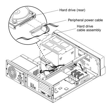
FIGURE 9-4 Removing and Replacing a Hard Drive (Ultra 5)
