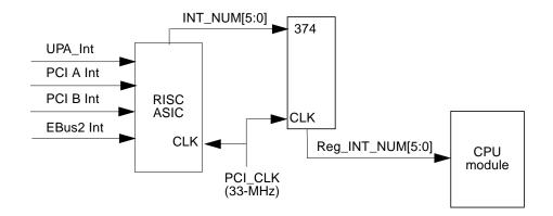
FIGURE C-16 Interrupt Scheme Block Diagram
