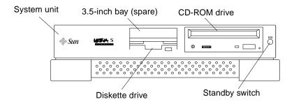
FIGURE 1-3 Ultra 5 System Unit Front View
