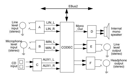
FIGURE C-15 Audio Circuit Functional Block Diagram
