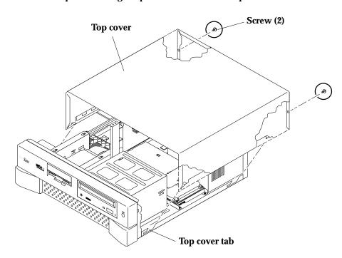
FIGURE 7-1 Removing and Replacing the Top Cover (Ultra 5)
