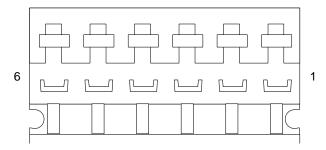
FIGURE 4-2 Power Supply Connector J20 Pin Configuration (Ultra 10 only)
