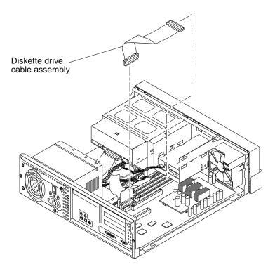
FIGURE 8-3 Removing and Replacing the Diskette Drive Cable (Ultra 5)
