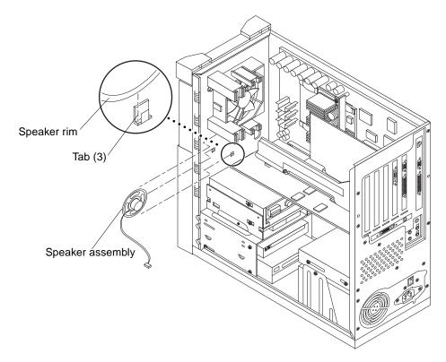
FIGURE 8-12 Removing and Replacing the Speaker Assembly (Ultra 10)
