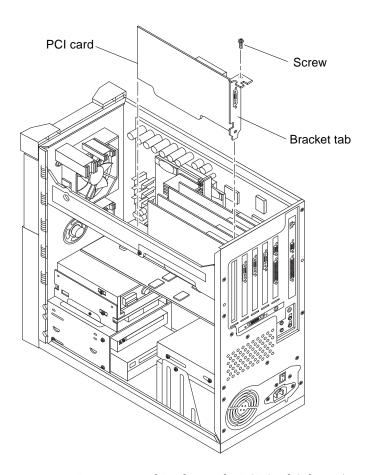
FIGURE 10-7 Removing and Replacing the PCI Card (Ultra 10)
