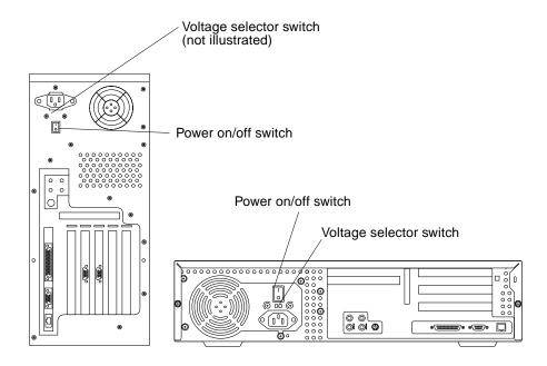
FIGURE 6-1 System Unit Power On/Off Switch
