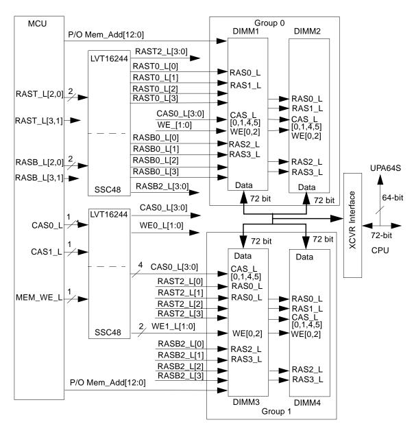
FIGURE C-10 Memory Interface Functional Block Diagram
