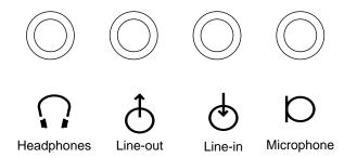
FIGURE B-8 Audio Connector Configuration
