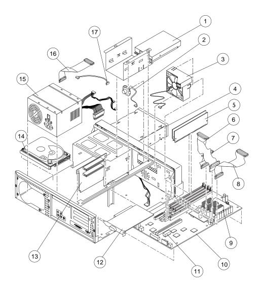
FIGURE 11-1 Ultra 5 Computer System Unit Exploded View
