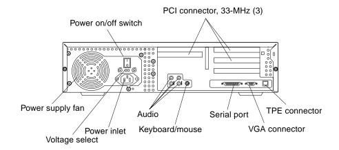
FIGURE 1-4 Ultra 5 System Unit Rear View
