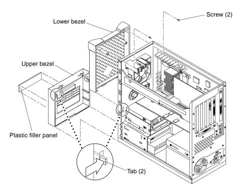
FIGURE 7-5 Removing and Replacing the Plastic Filler Panel (Ultra 10)
