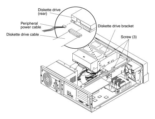
FIGURE 9-1 Removing and Replacing the Diskette Drive Part 1 (Ultra 5)
