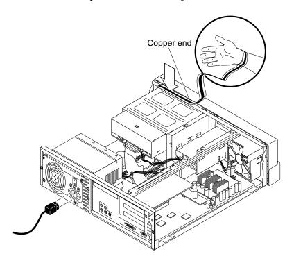
FIGURE 5-6 Attaching the Wrist Strap to the Chassis
