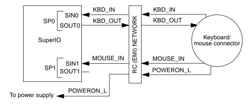
FIGURE C-11 Standard Serial Port Functional Block Diagram
