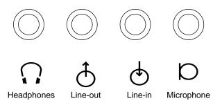
FIGURE B-7 Audio Connector Configuration
