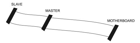
FIGURE C-4 EIDE Cable Labeling (With Secondary Hard Drive)
