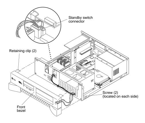
FIGURE 6-8 Removing and Replacing the Front Bezel
