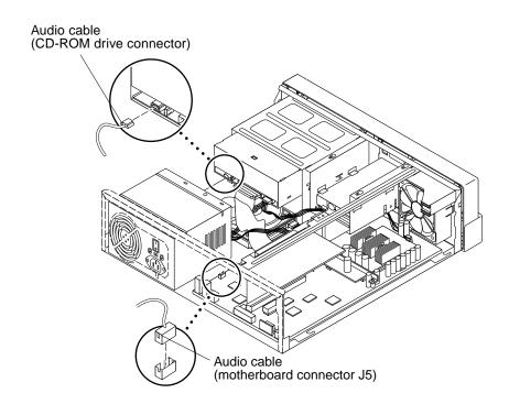
FIGURE 6-5 Removing and Replacing the Audio Cable
