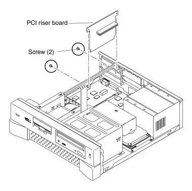
FIGURE 8-6 Removing and Replacing the PCI Riser Board
