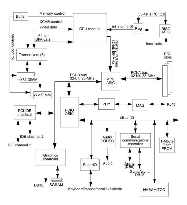
FIGURE C-1 System Functional Block Diagram
