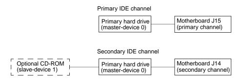
FIGURE A-4 Hard Drive Mirroring Configuration
