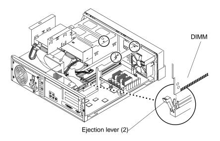
FIGURE 8-3 Removing and Replacing a DIMM
