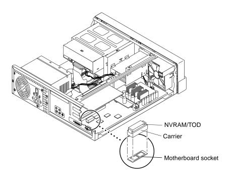
FIGURE 8-2 Removing and Replacing the NVRAM/TOD
