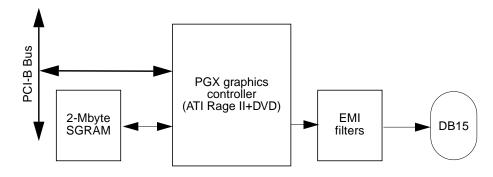
FIGURE C-7 PCI-Based Graphics Functional Block Diagram (PGX)
