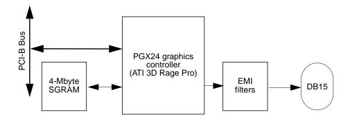
FIGURE C-8 PCI-Based Graphics Functional Block Diagram (PGX24)
