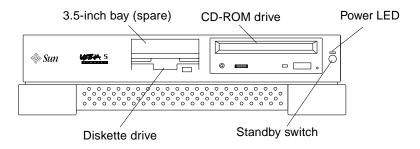
FIGURE 1-2 Ultra 5 System Front View
