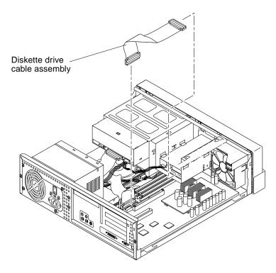
FIGURE 6-2 Removing and Replacing the Diskette Drive Cable Assembly
