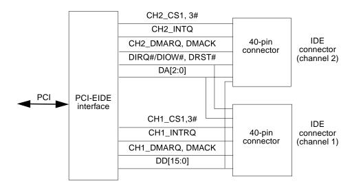
FIGURE C-3 EIDE Interface Functional Block Diagram
