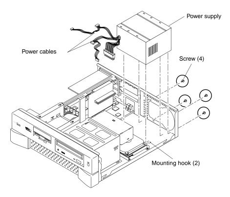
FIGURE 6-1 Removing and Replacing the Power Supply
