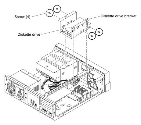
FIGURE 7-2 Removing and Replacing the Diskette Drive, Part 2
