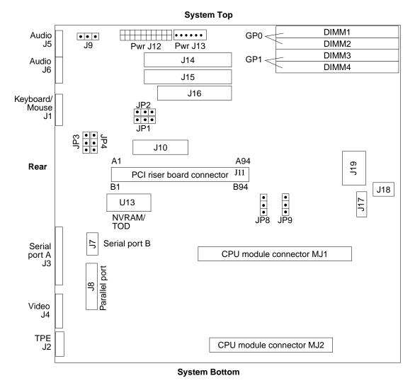
FIGURE C-16 Motherboard Block Diagram
