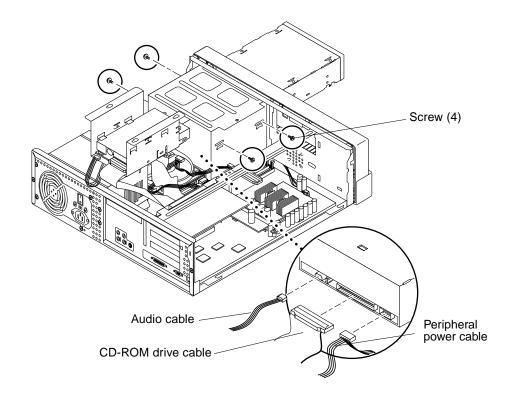
FIGURE 7-8 Removing and Replacing a CD-ROM Drive
