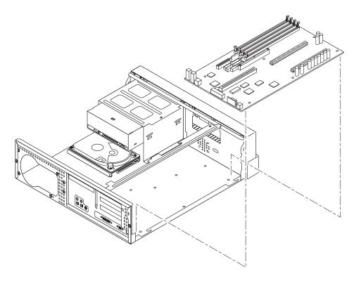
FIGURE 8-8 Removing and Replacing the Motherboard, Part 2
