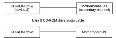
FIGURE A-1 CD-ROM Drive Cabling Configuration
