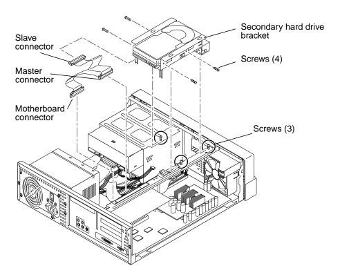
FIGURE 7-6 Installing a Secondary Hard Drive
