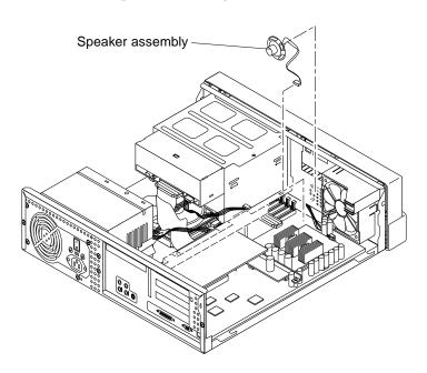
FIGURE 6-6 Removing and Replacing the Speaker Assembly
