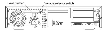
FIGURE 5-4 System Power Switch
