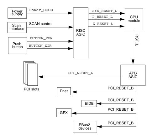
FIGURE C-10 System Reset Functional Block Diagram
