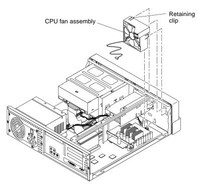
FIGURE 6-7 Removing and Replacing the CPU Fan Assembly
