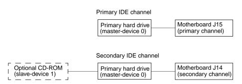
FIGURE 7-7 Hard Drive Mirroring Configuration
