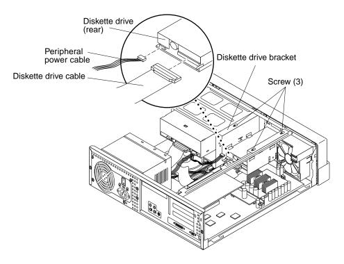
FIGURE 7-1 Removing and Replacing the Diskette Drive, Part 1
