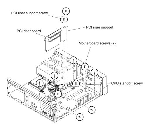
FIGURE 8-7 Removing and Replacing the Motherboard, Part 1
