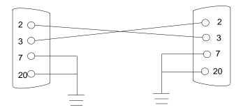
FIGURE 3-1 Setting Up a TIP Connection
