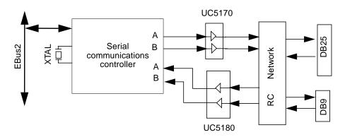
FIGURE C-12 Communications Controller Serial Ports Functional Block Diagram
