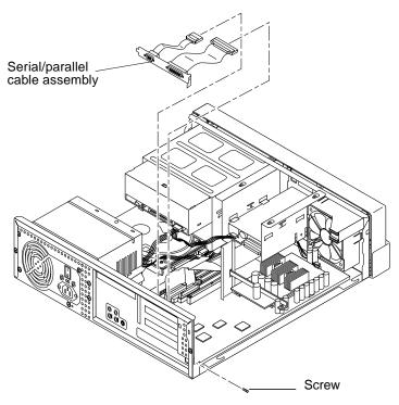
FIGURE 6-4 Removing and Replacing the Serial/Parallel Cable Assembly
