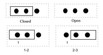
FIGURE 8-9 Identifying Jumper Pins
