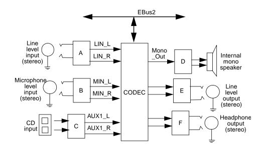
FIGURE C-14 Audio Circuit Functional Block Diagram
