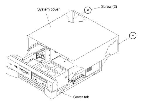
FIGURE 5-5 Removing the System Cover
