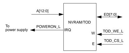
FIGURE C-13 NVRAM/TOD Functional Block Diagram
