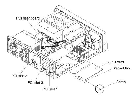
FIGURE 8-4 Removing and Replacing a PCI Card From PCI Slot 1 or 3
