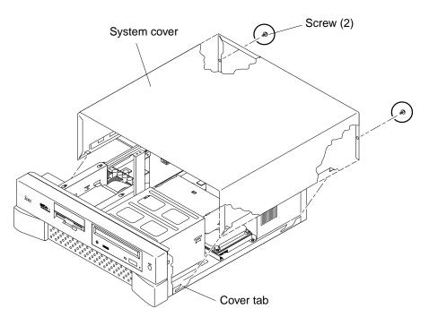
FIGURE 10-1 Replacing the System Cover
