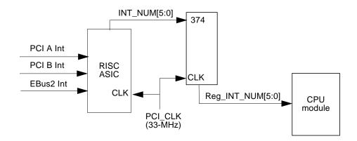
FIGURE C-15 Interrupt Scheme Block Diagram
