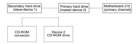
FIGURE C-6 Supported Ultra 5 Configuration (With Secondary Hard Drive)
