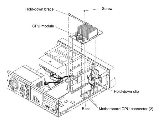
FIGURE 8-1 Removing and Replacing the CPU Module
