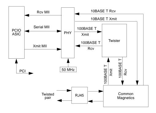
FIGURE C-2 10-/100-Mbit Ethernet Functional Block Diagram
