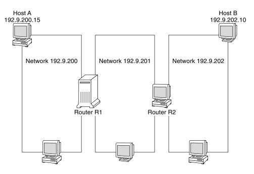
FIGURE 3-3 Three Interconnected Networks
