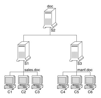
Clients C1, C2, and C3 would obtain their network information from server S1. Clients C4, C5, and C6 would obtain information from server S3. The resulting network is summarized in the following table. The table is a generalized representation of that network but does not resemble an actual network information map.
