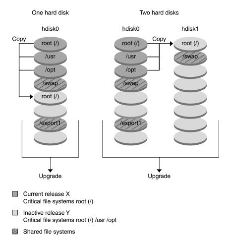
FIGURE 30–3 Creating an Inactive Boot Environment — Merging File Systems
