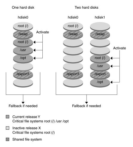
FIGURE 30–6 Activating an Inactive Boot Environment
