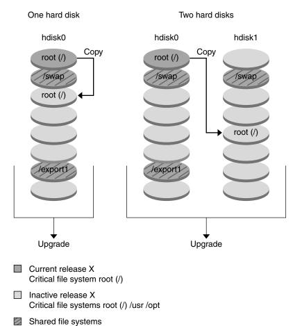
**FIGURE 30–1** Creating an Inactive Boot Environment — Copying root (/) to root (/)
