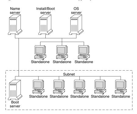
Figure 10–1 illustrates the servers that are typically used for network installation.
