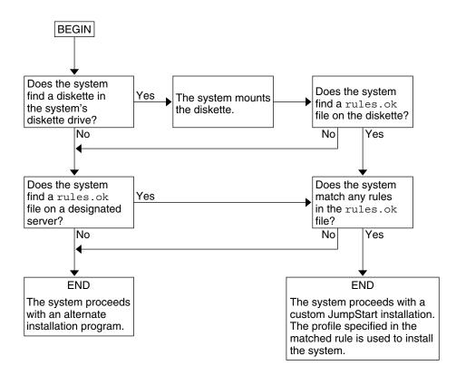
FIGURE 25-3 What Happens During a Custom JumpStart Installation
