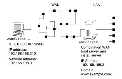
FIGURE 45-1 Sample Site for WAN Boot Installation
