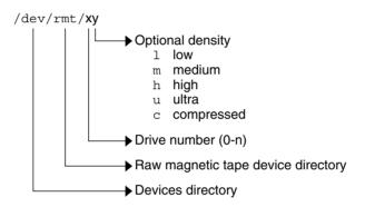
FIGURE 5-4 Logical Tape Device Names
