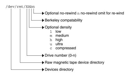
FIGURE 29-1 Tape Drive Device Names
