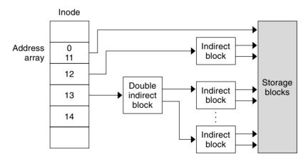
FIGURE 22–1 Address Chain for a UFS File System
