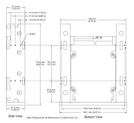
Figure 5. Internal DDS Drive with Rails—Dimensions
