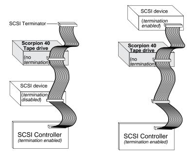
Figure 12. Two SCSI termination examples for internal Scorpion 40.
