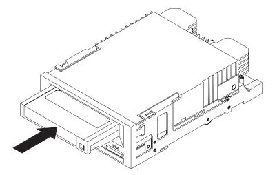
Figure 16. Loading a tape cartridge
