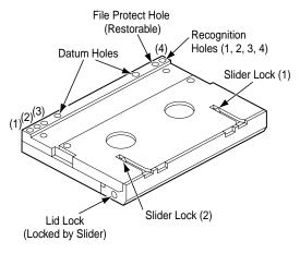
Figure 22. DDS-4 cartridge design features
