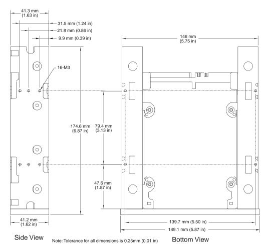
Figure 10. Mounting holes for internal Scorpion 40 in 5.25-inch configuration (with mounting brackets)
