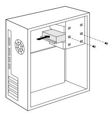
Figure 8. Mounting a drive
