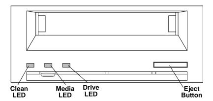
Figure 17. Location of Eject button and LEDs on internal Scorpion 40 (external drive is similar)
