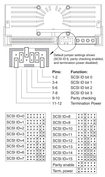
Figure 6. Jumper settings for internal Scorpion 40
