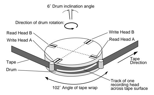
Figure 20. Four-head cylinder design
