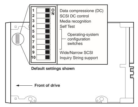
Figure 7. Dip-switch settings for internal Scorpion 40
