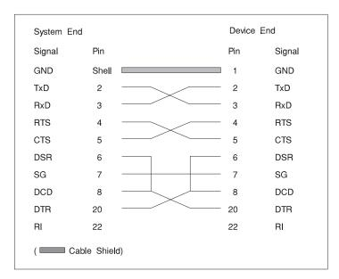
Figure B-3. Terminal/Printer Cable for EIA-232E Applications
