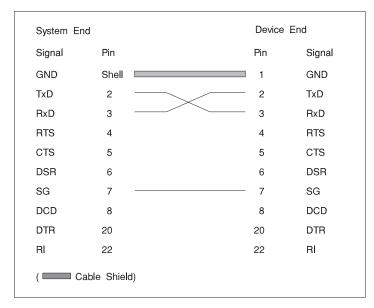
Figure B-1. Simple Terminal/Printer Cable for EIA-232E Applications
