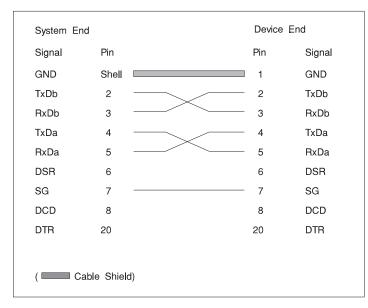
Figure B-2. Simple Terminal/Printer Cable for RS-422A Applications
