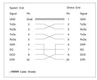
Figure B-4. Terminal/Printer Cable for RS-422A Applications
