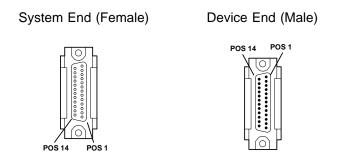
Figure A-1. Asynchronous Cable Connectors
