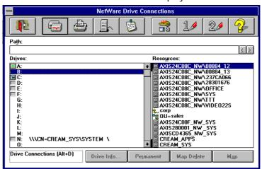
Note: o If the Show All Volumes parameter is set to yes, the individual discs are shown at the same level as SYS. Some applications will not run properly unless the data is stored at root level. To avoid such problems, assign a drive letter to that particular disc.
