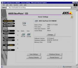
IDE Server - the icons displayed to the left represents all the units connected to the IDE bus listed as Master or Slave for each bus To display information on a particular device, simply click the corresponding icon:
