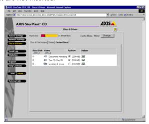
When an un-inserted mirrored disc is deleted it is removed from the list on this view.
