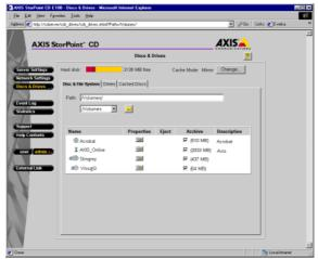
The Hard disk bar at the top of the page shows how much of the total hard disk space that is currently being used for archived copies and cached data. The free space available for archiving new discs is noted next to the bar. If you have more than one hard disk attached to the StorPoint CD+, the size of the largest disc that can be archived will be displayed below the bar. For more information about free hard disk space, go to the Statistics page.
