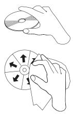
Compact discs are high-density media that must be handled with care and kept clean to ensure that they remain readable. Use the following precautions to ensure reliability:
