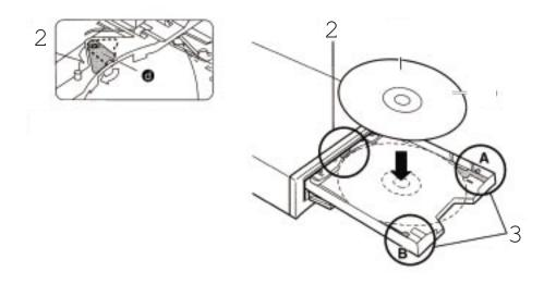
To load a compact disc into a horizontally mounted drive, do the following:
