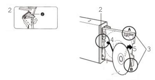
**Note:** The DVD-RAM drive must be in the horizontal position if you are using an 8cm disc.
