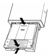
To load a DVD-RAM cartridge into a horizontally mounted drive, do the following:
