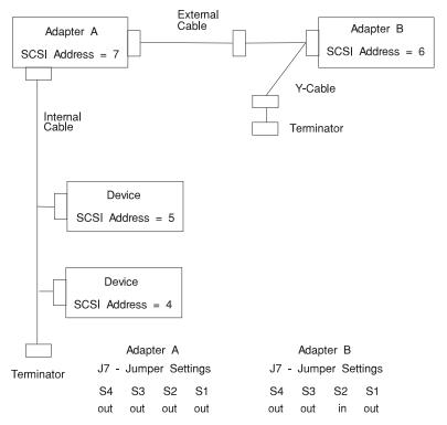
Figure C-3. Adapters Sharing Internal Devices
