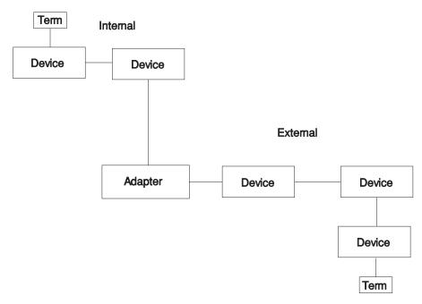
Figure C-2. SCSI Chain with Internal and External Devices
