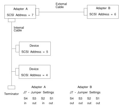
Figure C-4. Adapters Sharing Internal Devices with Simplified Cabling
