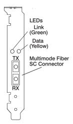
Figure 5-2. LEDs on the Gigabit Ethernet-SX PCI Adapter
