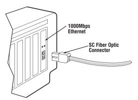
Figure 5-1. Connecting the Adapter to the Network
