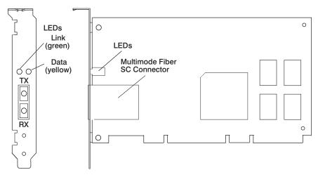
Figure 1-1. The Gigabit Ethernet-SX PCI Adapter
