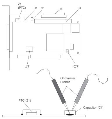
**Note:** Only the probe tips are touching the solder joints. Do not allow the probes to touch any other part of the component.
