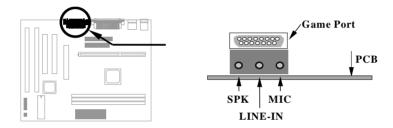
To fully utilize the audio functions, you may connect various peripheral devices that the audio chip supports. The following figure shows the different devices that you can connect.
