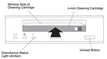
After the cleaning cartridge has been inserted, the remainder of the cleaning process is automatic. The tape drive:
