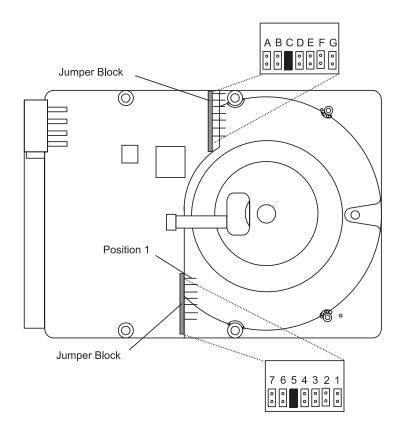
The previous illustration shows the pin positions on the 9.1 and 18.2 GB Ultra SCSI disk drives. Jumpers are required for positions C and 5.
