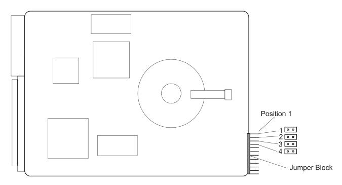
The previous illustration shows the pin positions on the 9.1, 18.2, 36.4, and 73.4 GB Ultra SCSI disk drives. No jumpers are required.
