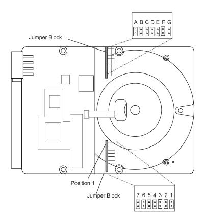
The previous illustration shows the pin positions on the 9.1, 18.2, 36.4, and 73.4 GB Ultra SCSI disk drives. No jumpers are required.
