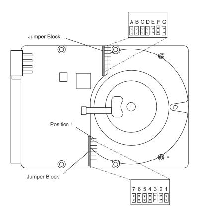
The previous illustration shows the pin positions on the 9.1, 18.2, and 36.4 GB Ultra SCSI disk drives. No jumpers are required.
