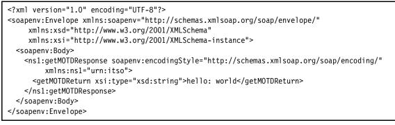
Figure 2-7 SOAP message from the Service Provider to the Service Requestor
