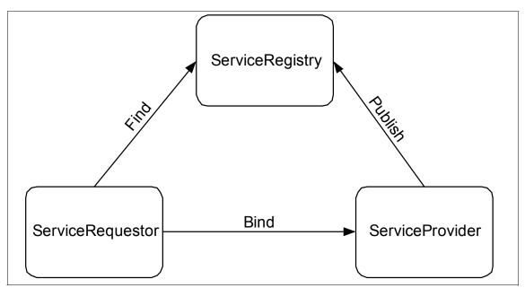
Figure 2-1 Elements of the Service Oriented Architecture (SOA)
