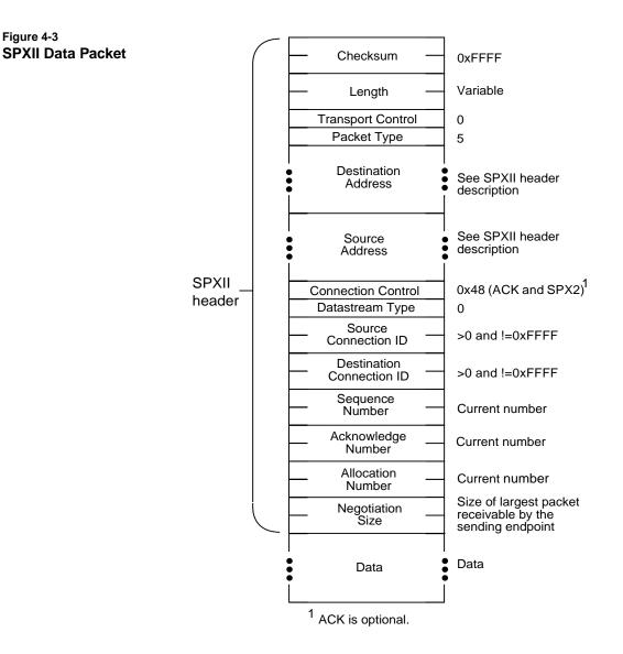
The Acknowledge Number field tracks the number of data packets the sender has received from the other endpoint. It is incremented on the reception of a packet and contains the value of the sequence number expected in the next data packet.
