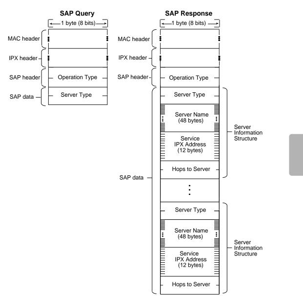
Figure 5-5 illustrates both SAP packet structures, query and response.
