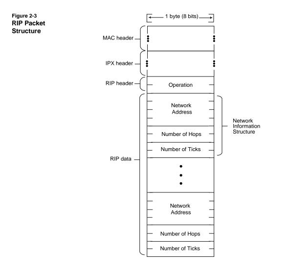
Figure 2-3 illustrates the RIP packet structure.
