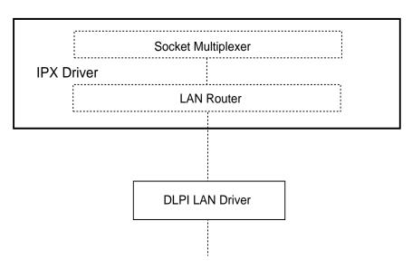
The socket multiplexer is the entity in the IPX software that delivers an IPX packet to the appropriate application (socket).
