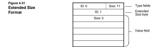
This ID subfield can contain one of 64 possible values. A value of 63 (111111 binary) indicates an Extended ID. When used, the extended ID immediately follows the Type field.
