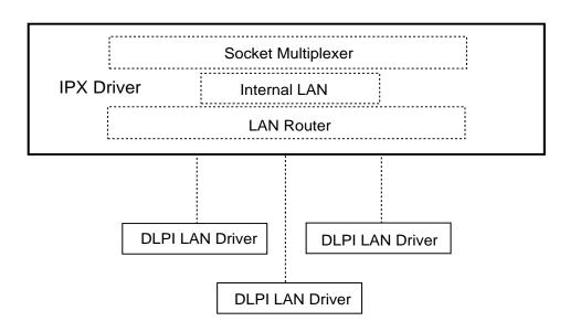
A LAN (Local Area Network) is a configured network in IPX. Each LAN (logical network) must be associated with a physical network and is limited to a single network frame type.
