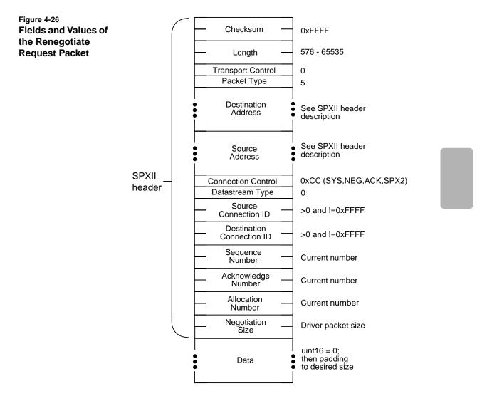
The header is followed by n bytes of data so that the packet size equals the driver packet size or smaller as required by negotiation retries. The first uint16 of the data must be zero (0) to indicate no optional information.
