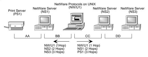
SAP agents use a split horizon algorithm to determine which SAP information to send to connected LANs. This algorithm ensures that the SAP agent does not broadcast information back to the same SAP agent from which the information was obtained.
