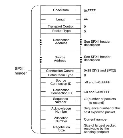
Figure 4-5 Fields and Values of an SPXII NAK Packet
