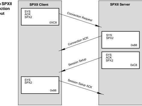
If the client does not receive a Session Setup packet within a specific time period, a session setup timeout occurs. This timeout will abort the connection establishment and notify the application of the failure. The time period begins with the reception of the Connection ACK. The SPXII driver uses the watchdog timer, which has a default of 60 seconds.
