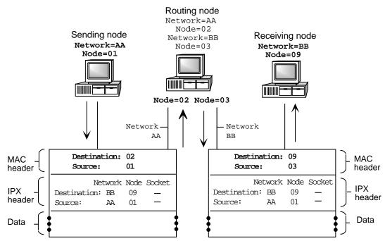
In our example above, the sending node resides on Network AA and the receiving node resides on Network BB. A NetWare server is the router on Network AA with the shortest route to Network BB.
