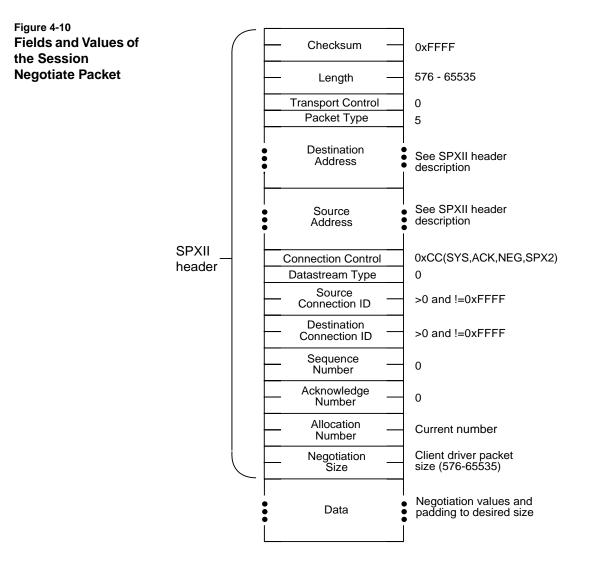
The header is followed by *n* data bytes. The client SPXII driver pads the Data field so that the packet size equals the maximum packet size that both the server driver and client driver can support.
