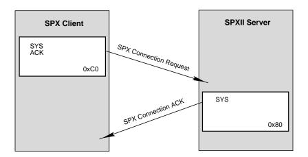
The client issues an SPX Connection Request (which does not have the SPX2 bit set).
