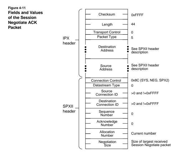
The server uses the Length field in the IPX header to determine the size of the Session Negotiate packet. It then uses this value to set the value of the Negotiation Size field in the Session Negotiate ACK packet. If the server receives multiple Session Negotiate packets (because of delayed packets or lost ACKs), the server always sets the Negotiation Size field to the value of the largest received Session Negotiate packet.
