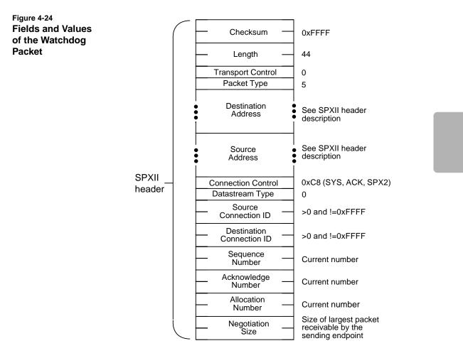
A data ACK can be "piggy-backed" on a watchdog packet by increasing the Acknowledge number to reflect all packets received (all packets up to but not including the acknowledge number have been received).
