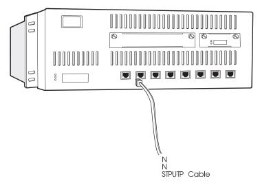
Connecting the UTP/STP Cable to an ATM Switch
