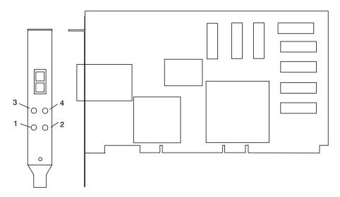
The LEDs on the TURBOWAYS 622 PCI MMF ATM Adapter provide information about the adapter's operation status. The LEDs are visible through the adapter's mounting bracket and, when lit, indicate the following conditions:
